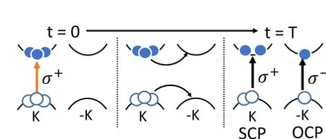
Valley relaxation measurement: Pump pulse excites at t=0 and probe light of same (SCP) or opposite (OCP) C-polarization is transmitted at t=T.
